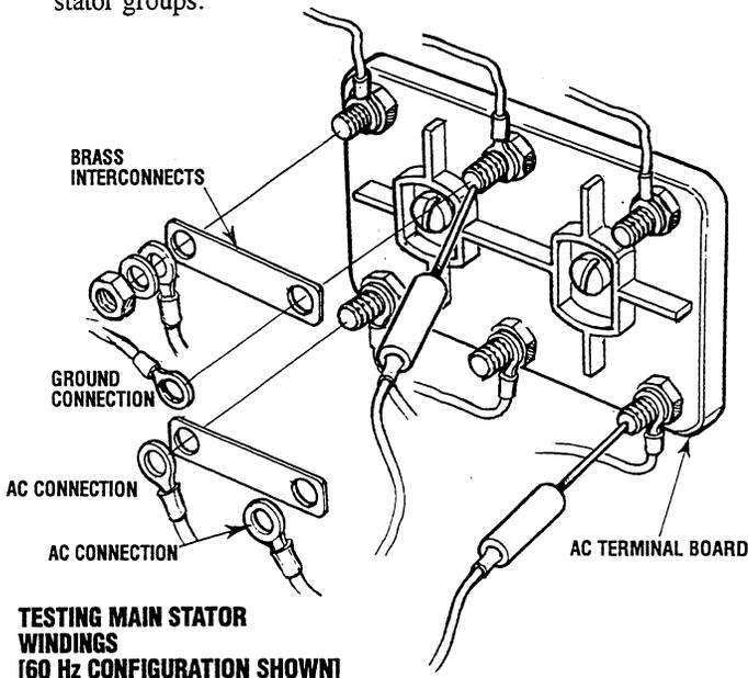
**TESTING MAIN STATOR WINDINGS [60 Hz CONFIGURATION SHOWN]**
