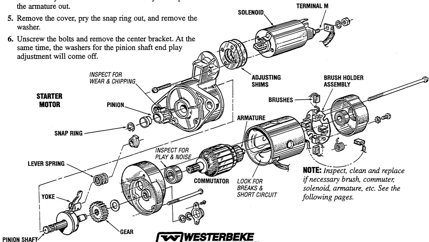
**NOTE:** Inspect, clean and replace if necessary brush, commutator, solenoid, armature, etc. See the following pages.
