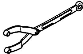
**CRANKSHAFT FRONT OIL SEAL INSTALLER**
