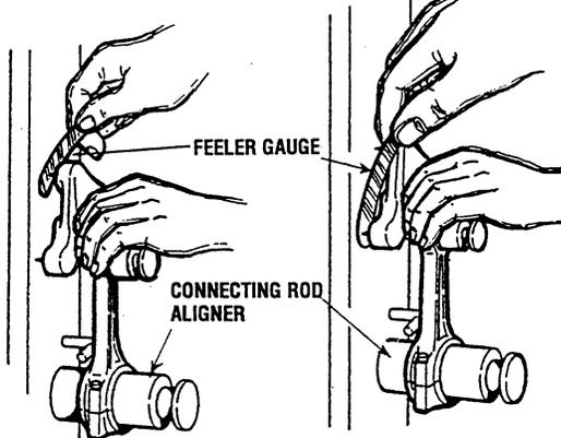
**CONNECTING ROD TWIST LIMIT** 0.004in (0.1mm)
