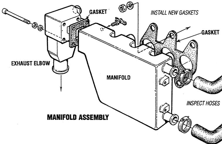
1. Remove the exhaust elbow from the manifold. Scrape off and discard the old gasket. Inspect the exhaust elbow for corrosion and damage, replace if necessary.
