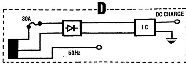
**NOTE:** The battery charging circuit is totally separate from the AC output of the generator. The generator output affects the circuit's output, but not the reverse.
