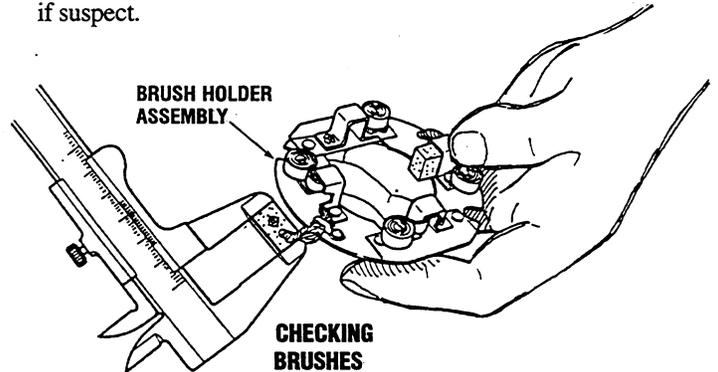
3. Check for insulation between the positive brush holder and holder base. If poorly insulated, replace the holder assembly. Also check the brush holders for proper staking.
