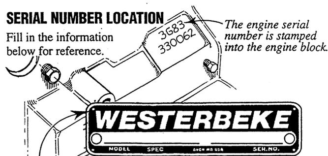
The engine model number and serial number are printed on a decal on the engine manifold.
