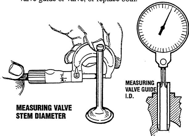
**MEASURING VALVE STEM DIAMETER**
