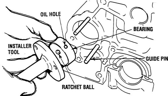
2. Mate the ratchet ball of the bearing in the oil hole of the rear bearing and install the bearing in the bearing installer.
