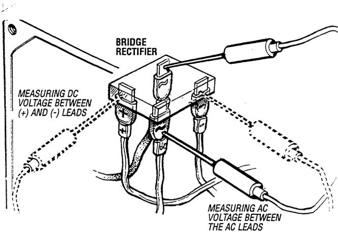
Normal DC voltage running out of the rectifier (in volts DC) is measured across the two DC connections of the bridge rectifier, that is + and - as illustrated.
