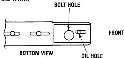
6. Tighten the rocker arm shaft bolts (4 bolts) uniformly and then to the specified torque.
