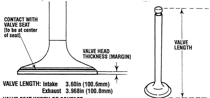
VALVE LENGTH: Intake 3.60in (100.6mm)
