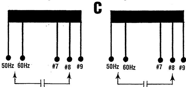
**⚠ WARNING:** Make certain the insulating covers on the unused leads are in place and are **NOT** in contact with each other or in contact with the generator's housing.
